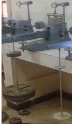
Fig. 5. Compressibility test on a soil sample studied during its execution.
