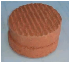
Fig. 6. Soil sample studied after the direct shear test.
