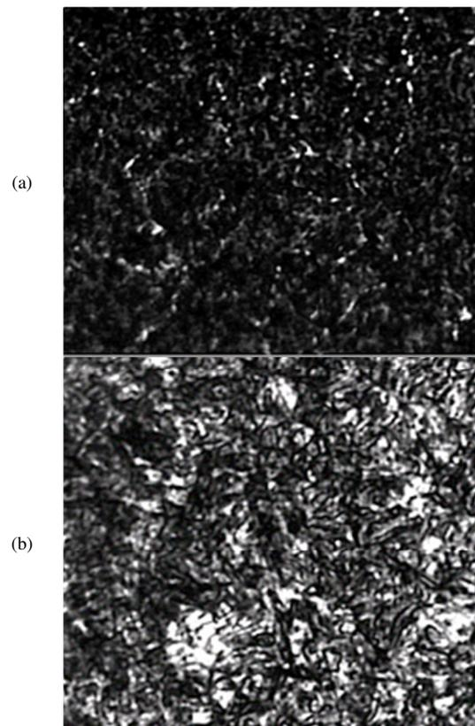
Fig. 2. Micrograph after carburizing at  $900^\circ\text{C}$  and quenching for 1h. (a) Surface zone, (b) inner area.
