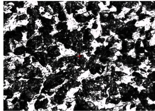
Fig. 1. Microstructure of the steel before the carburizing treatment.
