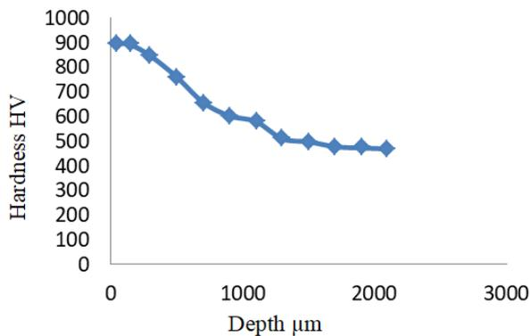
Fig. 6. Hardness of steel carburized at 900°C for 2h.
