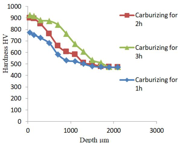
Fig. 8. Hardness of steel carburized at 900°C for 1, 2, and 3 hours.
