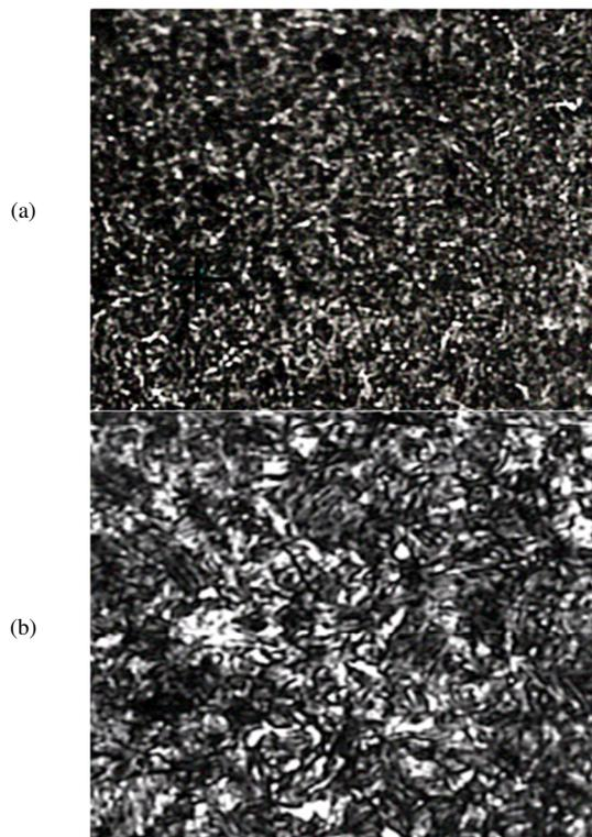
Fig. 3. Micrograph after carburizing at 900C° and quenching for 2h. (a) Surface zone,(b) inner area.
