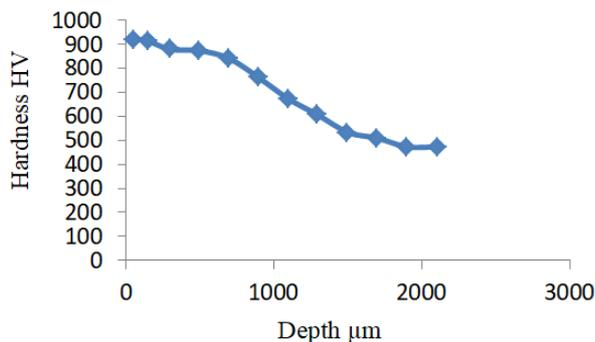
Fig. 7. Hardness of steel carburized at 900°C for 3h.
