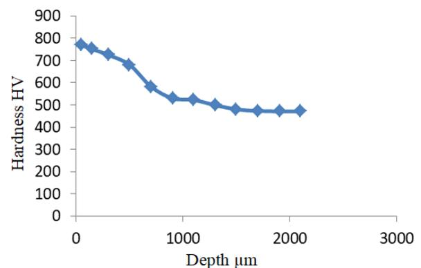
Fig. 5. Hardness of steel carburized at 900°C for 1h.
