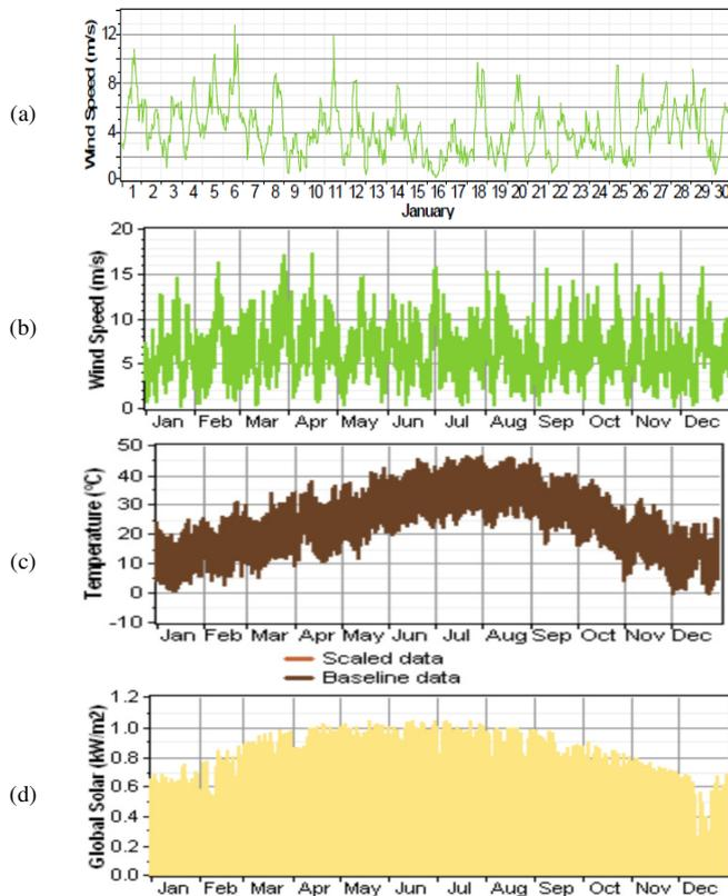
Fig. 3. Seasonal variations of the amount of renewable energy in the Algerian Sahara: (a) Wind speed in Tindouf, (b) wind speed in Adrar, (c) temperature changes in Adrar, (d) solar energy in Adrar.
