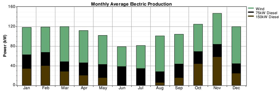
Fig. 7. Power produced by the system during the year. Environmental rating analysis.
