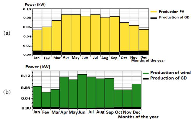
Fig. 1. Yearly produced power from the system: (a) PV and GD, (b) WT and DG.
