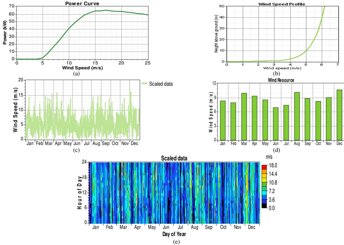
Fig. 6. Characteristics of the wind turbine: (a) Property of the power for the wind turbine used, (b) wind speed according to the height of the turbine used, (c) changes in wind speed during the year, (d) average wind speed during the year, (e) DMAP for wind speed changes.
