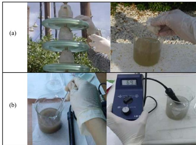
Fig. 6. (a) Collection of pollutants on site (b) Stirring and measuring the conductivity of the solution
