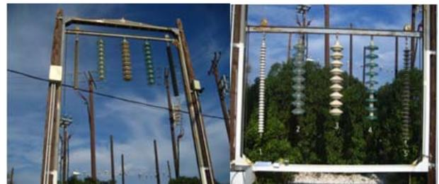
Fig. 4. The ESDD arch with the specimen insulators in the upper and lower position
