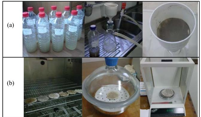
Fig. 7. (a) Solutions into labeled bottles, forced filtering with the help of a water vacuum pump and residuum on the filter paper (b) Filters in the drying oven, desiccator and precision scale
