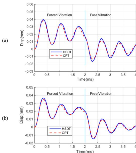
Fig. 3. The deflection response at the central plate. Cases (a) 1, (b) 2.
