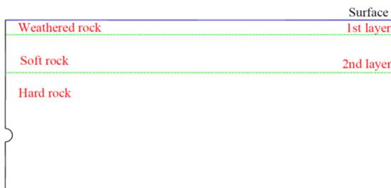
Fig. 6. A computational model for inhomogeneous rock mass.
