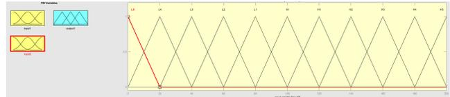
Fig. 6. Input 2 (actual voltage) membership functions.
