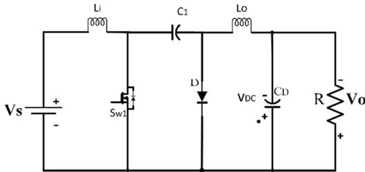
Fig. 4. CUK converter circuit.
