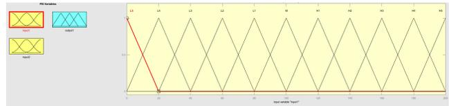
Fig. 5. Input 1 (ref. voltage) membership functions.
