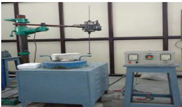
Fig. 1. Experimental setup for reinforcement using stir casting.
