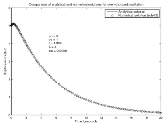
Fig. 2. Comparison between analytical (solid line) and numerical (circles) solutions for over-damped nonlinear response
