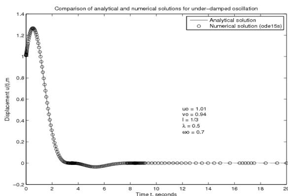
Fig. 4. Comparison of analytical and numerical solutions for under-damped oscillation
