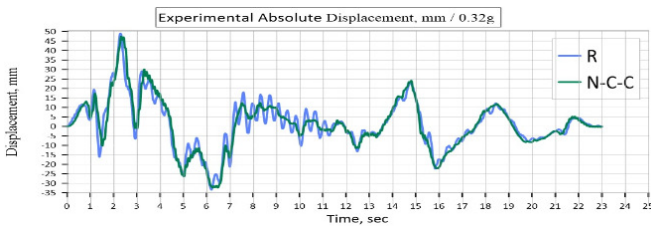
Fig. 21. Time-displacement of R and N-CI-C models with 0.32g excitation.
