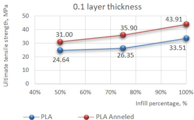
Fig. 2. Ultimate tensile strength variation of 0.1 layer thickness for varying infill percentage.
