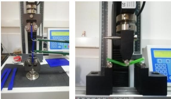
Fig. 1. Tensile and flexural sample testing on the Lloyd LRX Plus Testing Machine.
