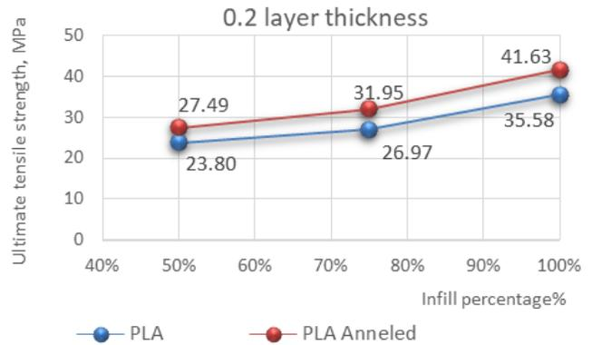
Fig. 4. Ultimate tensile strength variation of 0.2 layer thickness for varying infill percentage.
