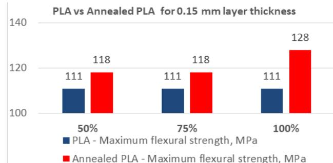
Fig. 6. Maximum flexural strength comparison between PLA and annealed PLA for 0.15mm layer thickness.
