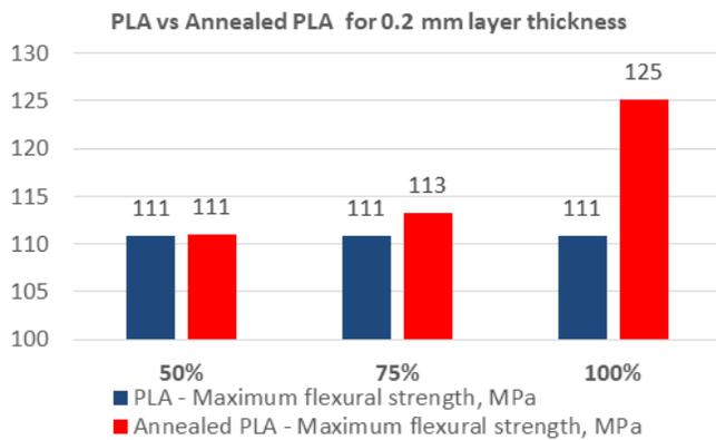
Fig. 7. Maximum flexural strength comparison between PLA and annealed PLA for 0.2mm layer thickness.
