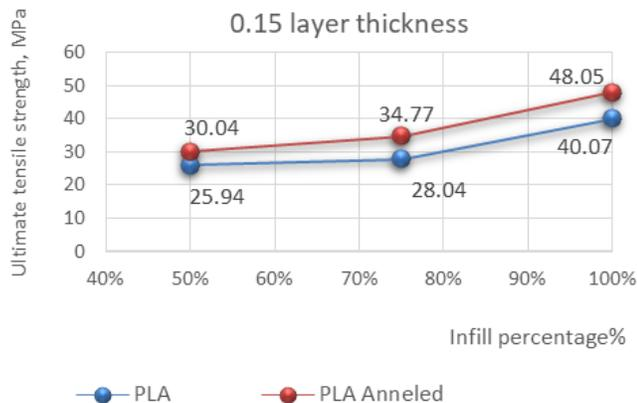
Fig. 3. Ultimate tensile strength variation of 0.15 layer thickness for varying infill percentage.
