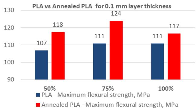
Fig. 5. Maximum flexural strength comparison between PLA and annealed PLA for 0.1mm layer thickness.
