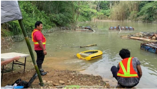
Fig. 11. Navigation system actual testing in a mining tailing pond.
