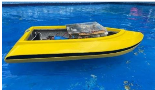
Fig. 10. Buoyancy and stability test of the mini-boat.
