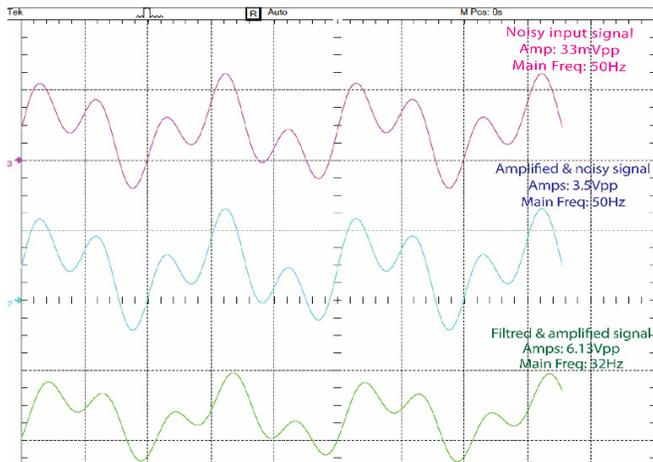
Fig. 10. Amplified and filtered output signal.
