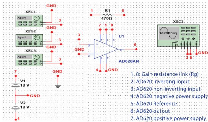
Fig. 5. Pre-amplification circuit.
