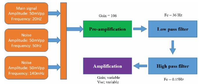
Fig. 3. Stages of the acquisition card.
