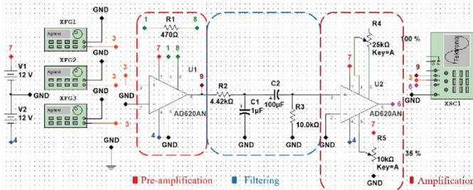
Fig. 9. Diagram of ECG signal detecting, amplification, and filtering.
