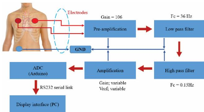
Fig. 1. ECG data acquisition system.
