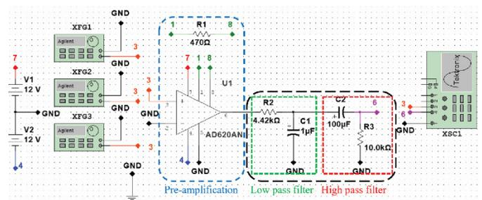
Fig. 7. Pre-amplification and filters.
