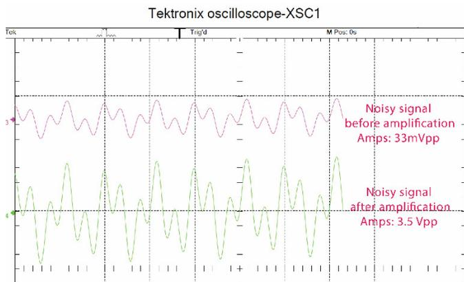
Fig. 6. Pre-amplification block results.
