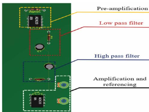
Fig. 2. ECG amplifier, high-and low-pass filters.
