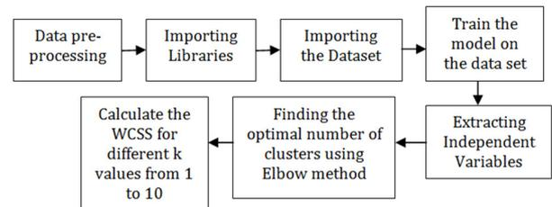
Fig. 7. The process of finding the clusters.
