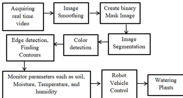
Fig. 1. Block diagram of the proposed work.
