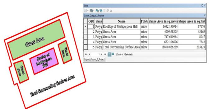
Fig. 5. Calculation of the areas of digitized rooftop and plain surface catchments using ArcGIS.
