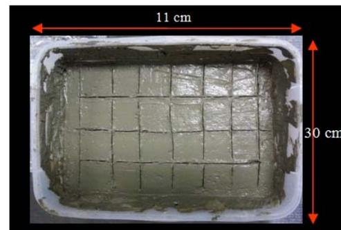
Fig. 2. Remolded soil bed with grids marked out for the measurements
