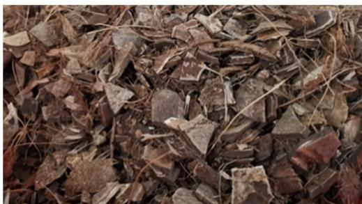
Fig. 2. Torrefied coconut shells.
