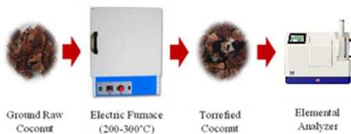
Fig. 1. Torrefaction experimental setup.
