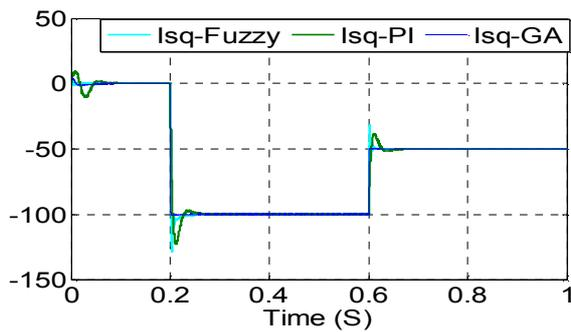
Fig. 11. The quadrature current of the stator (A).
