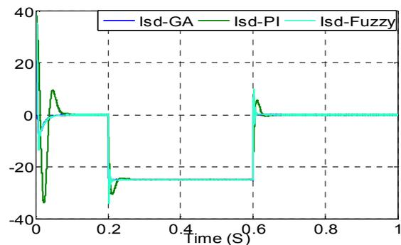
Fig. 10. The direct current of the stator (A).
