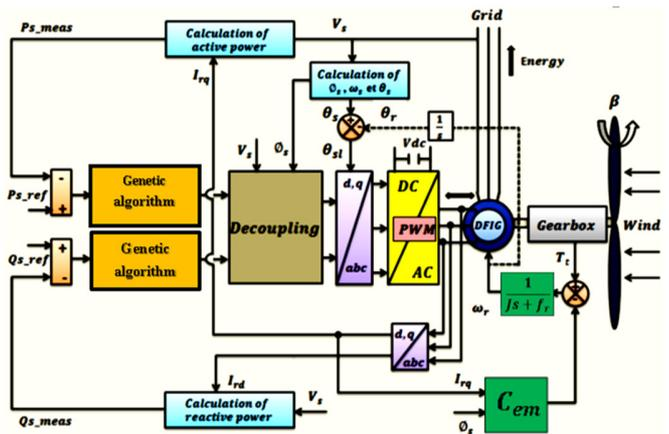
Fig. 5. Global block diagram of the command of the GA based on DFIG.
