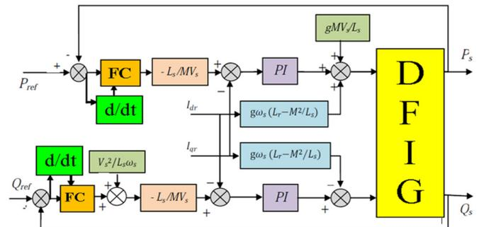
Fig. 2. Indirect closed loop fuzzy control diagram.
