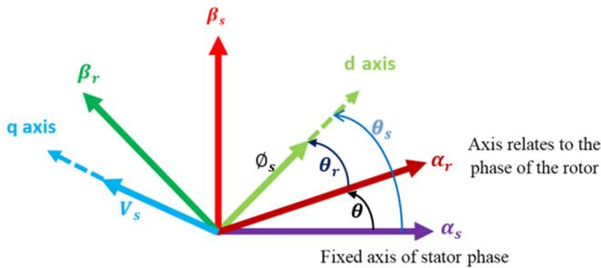
Fig. 1. Direction of stator voltage and flux.
