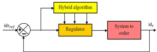
Fig. 4. Principle of optimization by genetic gradient or simplex algorithm.
