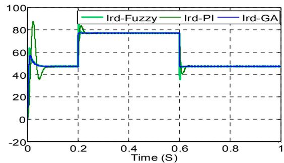
Fig. 8. The direct current of the rotor (A).
