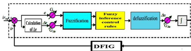
Fig. 3. Block diagram of the fuzzy controller.
