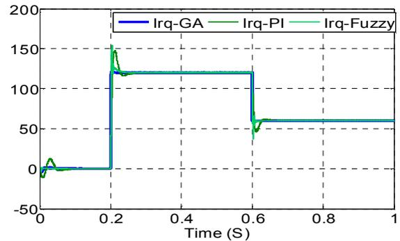
Fig. 9. The quadrature current of the rotor (A).
