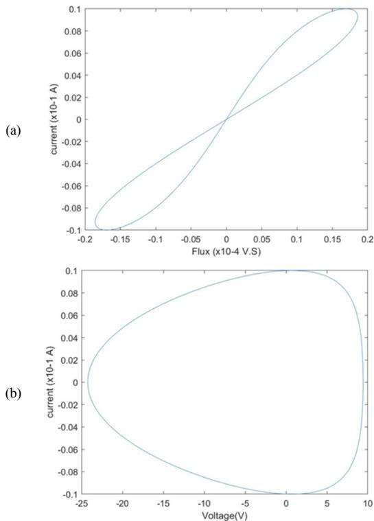
Fig. 3. (a) Flux and current pinch hysteresis loop, (b) variation of current versus voltage.
