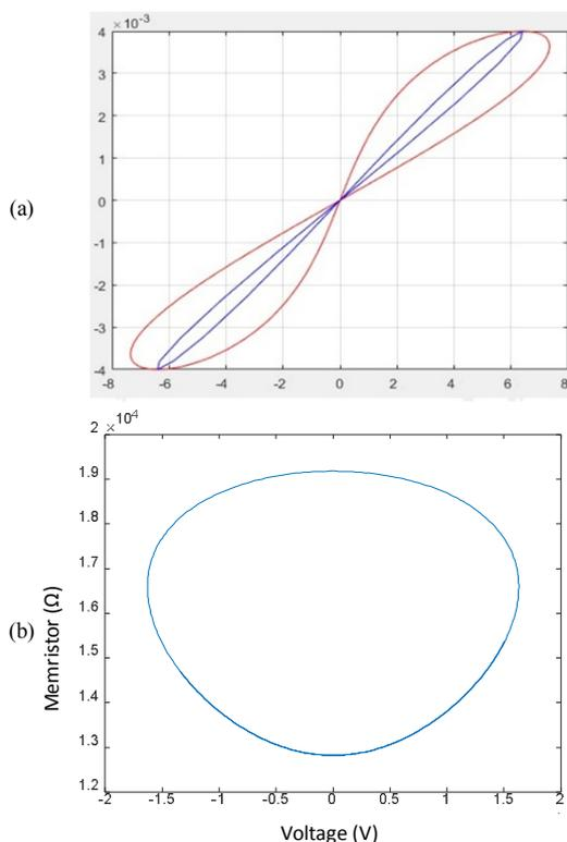
Fig. 1. (a) Pinched hysteresis loop appearing between current and voltage for sinusoidal input with frequency  $f=10\text{Hz}$  (green),  $50\text{Hz}$  (red), (b) Variations of memristif values versus voltage.
