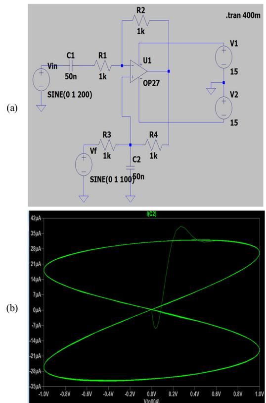
Fig. 4. Memcapacitor emulator.
