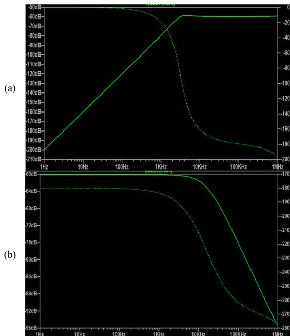
Fig. 6. Frequency simulations of emulators: (a) memcapacitor, (b) meminductor.
