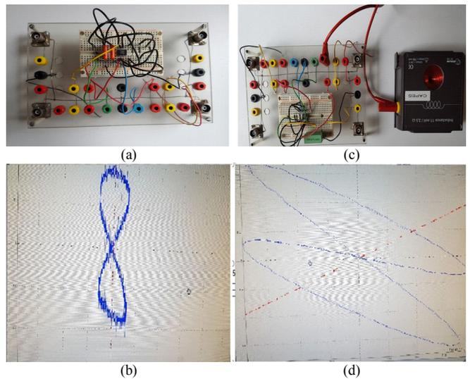
Fig. 8. Experimental implementation and results: (a) (b) Memcapacitor, (c) (d) Meminductor.
