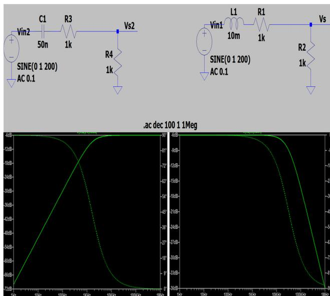
Fig. 7. Equivalent circuit filters and simulation results.
