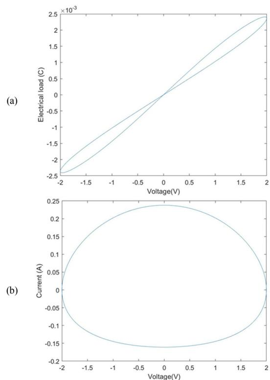
Fig. 2. (a) Voltage and electric load pinch hysteresis loop, (b) variation of current versus voltage.
