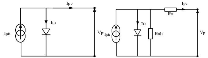
Fig. 1. Electrical model of a solar cell.
