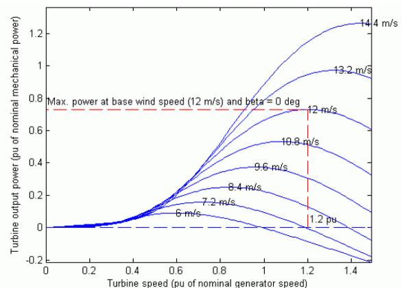
Fig. 5. Turbine power characteristics with wind as parameter.
