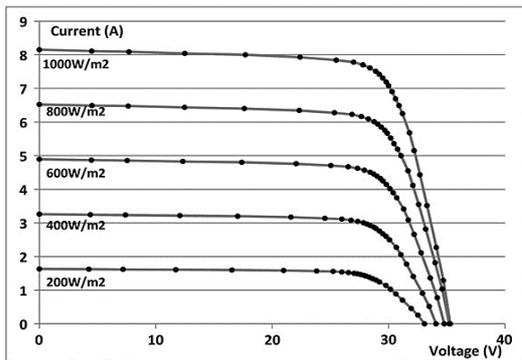
Fig. 3. I-V Characteristics of PV at constant temperature of 25°C and different irradiances.
