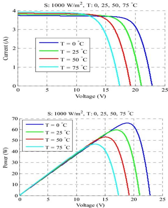
Fig. 2. I-V characteristics at different temperature and constant irradiance of 1000W/m<sup>2</sup>.
