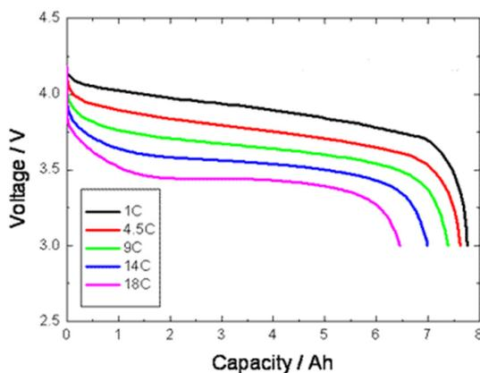
Fig. 7. Charge and discharge characteristics of the battery.
