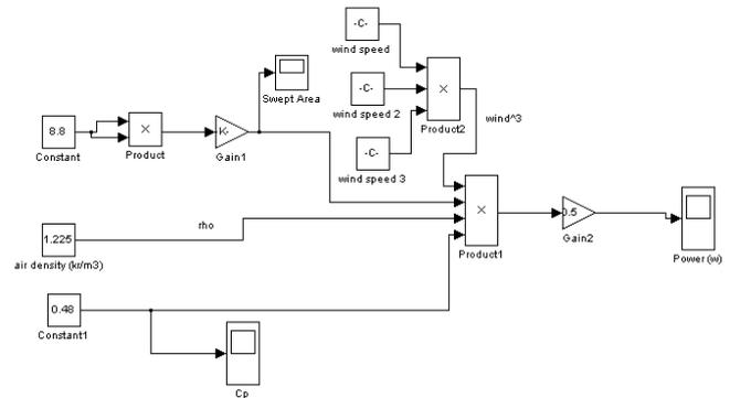
Fig. 4. Simulink mathematical model of the wind turbine.
