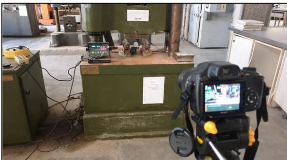
Fig. 8. Geopolymer prisms while testing.
