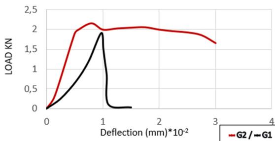
Fig. 7. Load deflection curve at 28 days.
