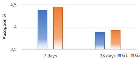
Fig. 2. Water absorption of G1 and G2 mixes.
