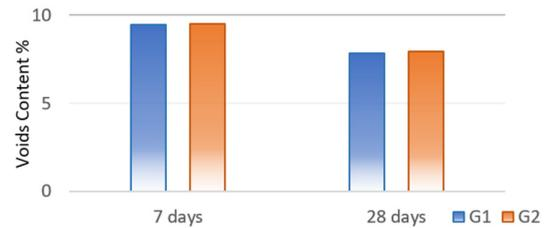
Fig. 3. Void Content % of G1 and G2 mixes.
