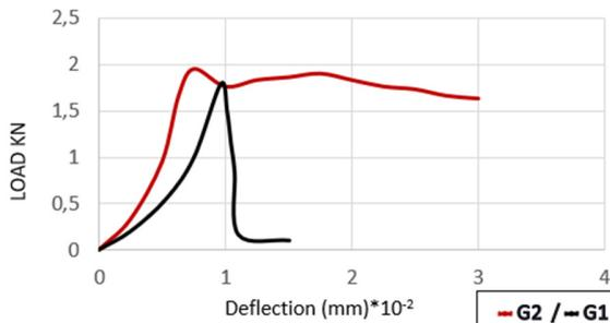
Fig. 6. Load deflection curve at seven days
