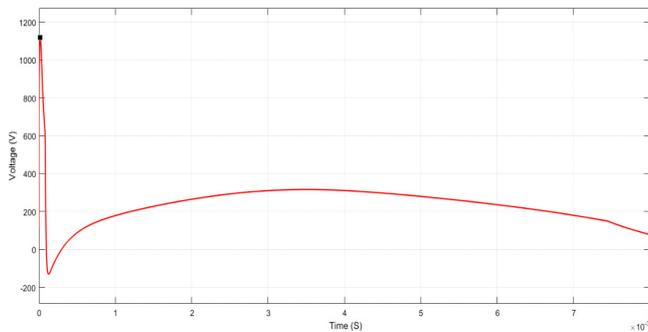
Fig. 6. Waveform of the protection voltage across the AC load after the installation of class I and II SPDs.
