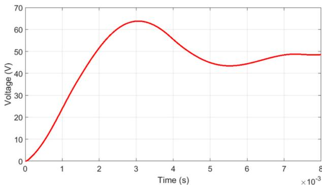
Fig. 7. Waveform of protection voltage across the DC load after the SPD installation.
