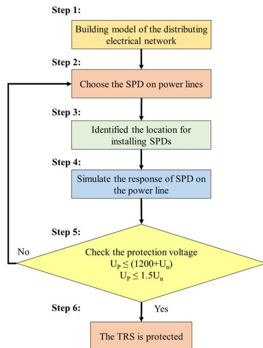
Fig. 2. Procedure for testing and installing SPDs.
