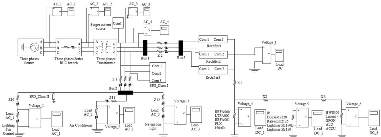
Fig. 3. Model of the distribution network in Matlab-Simulink.
