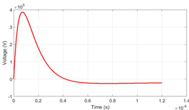
Fig. 4. Waveform of protection voltage across the AC load when SPD is not installed.
