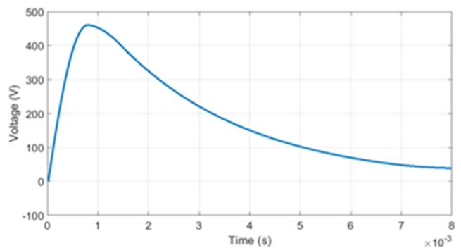
Fig. 5. Waveform Protection voltage across DC load after SPD installation.
