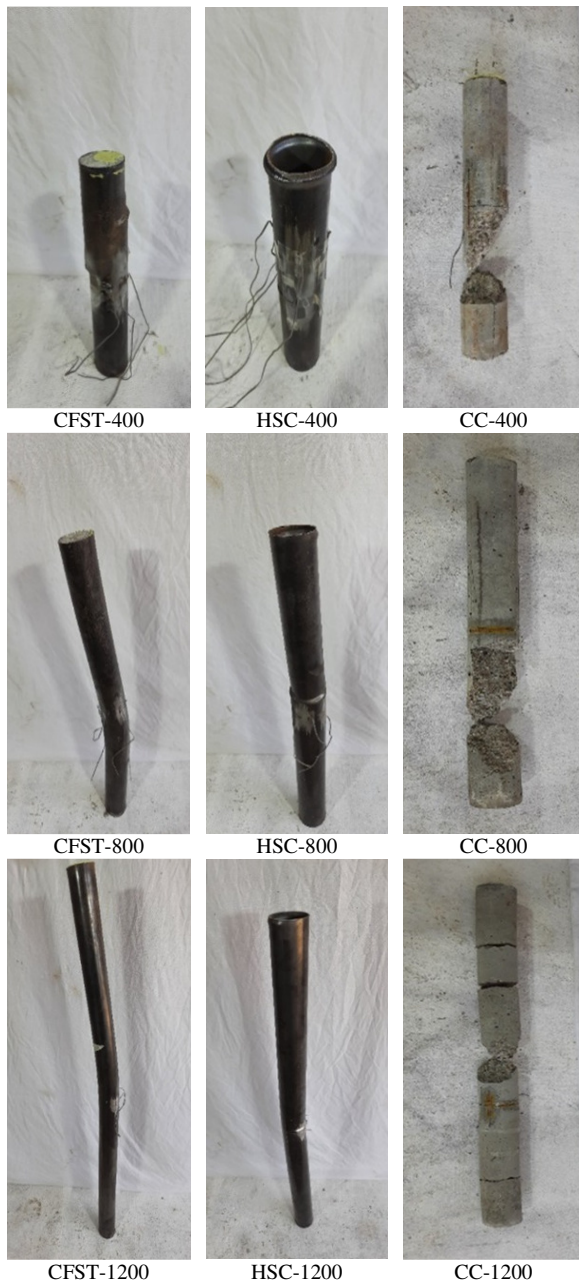
Fig. 19. Failure modes of the tested specimens.
