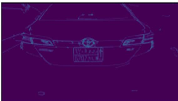
Fig. 9. The output of the morphological gradient.
