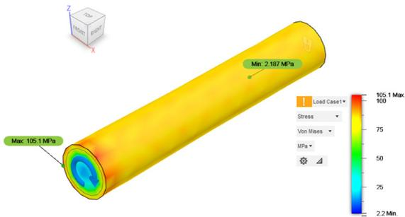
Fig. 1. Example of a shaft (10mm diameter × 60mm) simulated with a torque applied on the face (SF).
