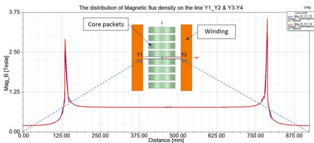
Fig. 5. Magnetic flux density along the lines Y1-Y2 and Y3-Y4 on the surface of a core packet.
