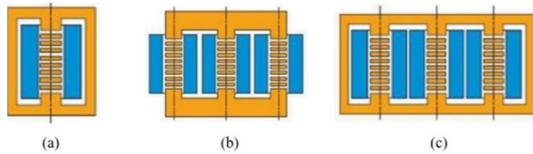
Fig. 1. Modeling of the shunt reactor: (a) single-phase, (b) 3-phase 3-limbed core, (c) 3-phase 5-limbed core [6].
