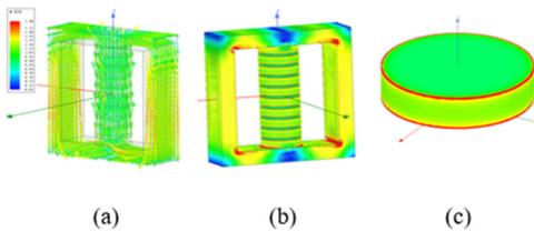
Fig. 4. The magnetic flux density on the magnetic circuit and iron core packets.
