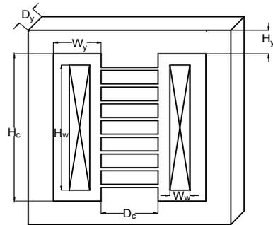
Fig. 2. Model of the shunt reactor.
