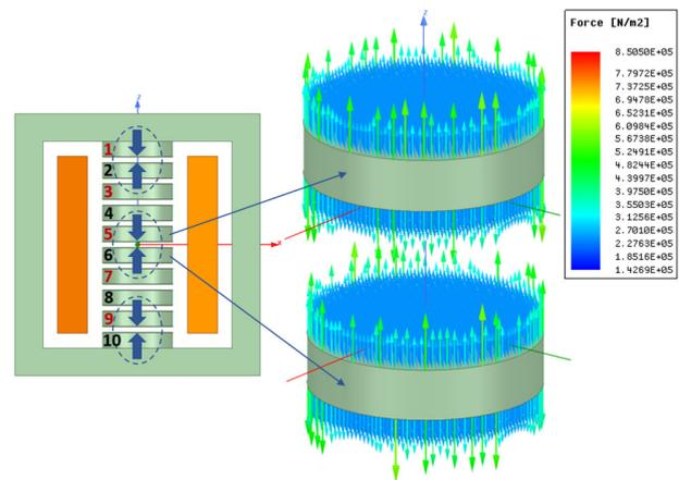
Fig. 6. Distribution of the force density on the surface of the core packets.
