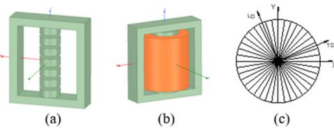
Fig. 3. 3D model of the single-phase SR and the radially laminated silicon steels.
