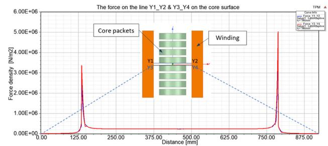
Fig. 7. Distribution of force density along the lines Y1-Y2 and Y3-Y4 on the core surface.
