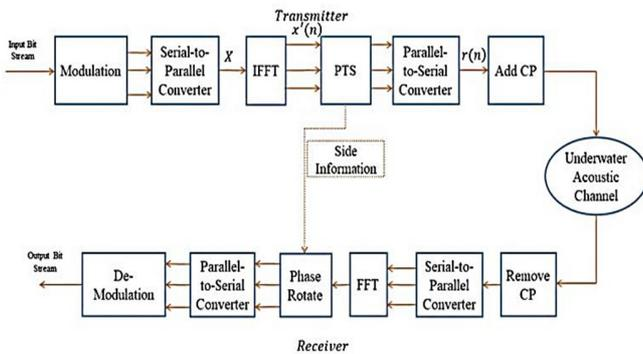
Fig. 1. Block diagram of the system model.
