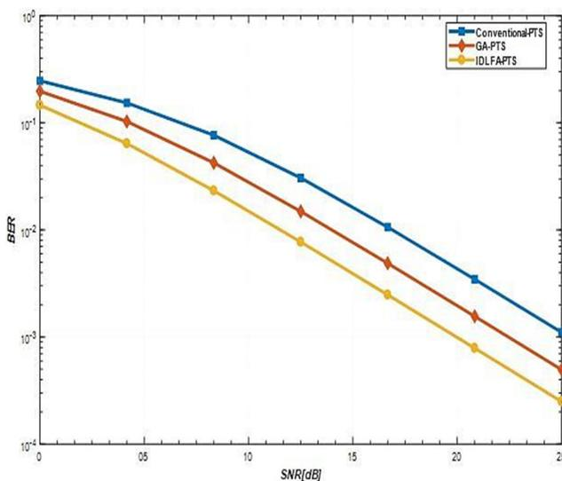
Fig. 5. Comparison of proposed IDFLA-PTS, GA-PTS, and conventional-PTS in terms of BER.
