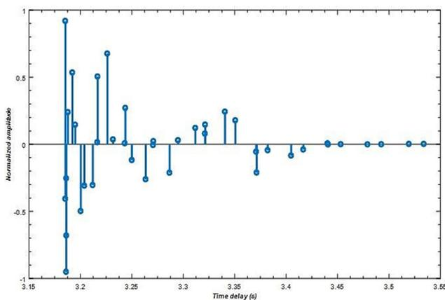
Fig. 7. Channel impulse response of the underwater tank with the IDFLA-PTS algorithm.
