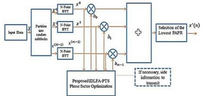
Fig. 2. Block diagram of the proposed IDFLA-PTS.
