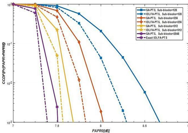
Fig. 4. PAPR comparison of IDFLA-PTS, GA-PTS, and exact IDFLA-PTS.
