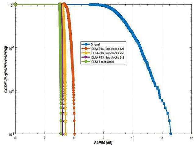
Fig. 3. PAPR comparison of IDFLA-PTS, exact IDFLA-PTS, and original OFDM signal.
