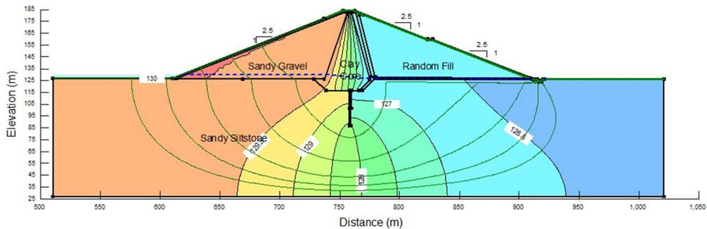
Fig. 5. Flow net of the selected section at minimum reservoir level (130m).
