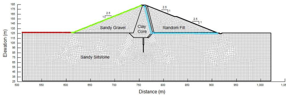
Fig. 2. Mesh formation for the selected non-homogeneous section.
