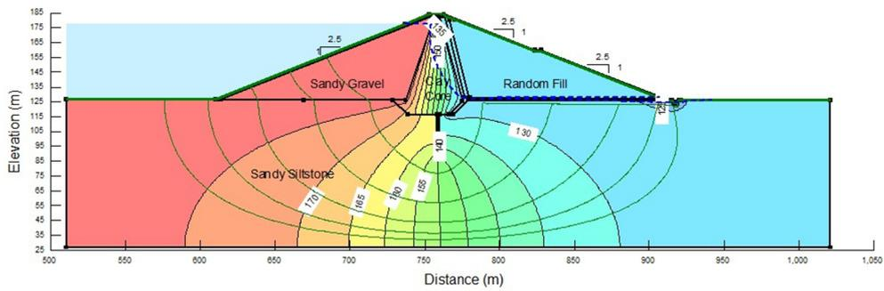
Fig. 3. Flow net of the selected section at maximum reservoir level (177.5m).
