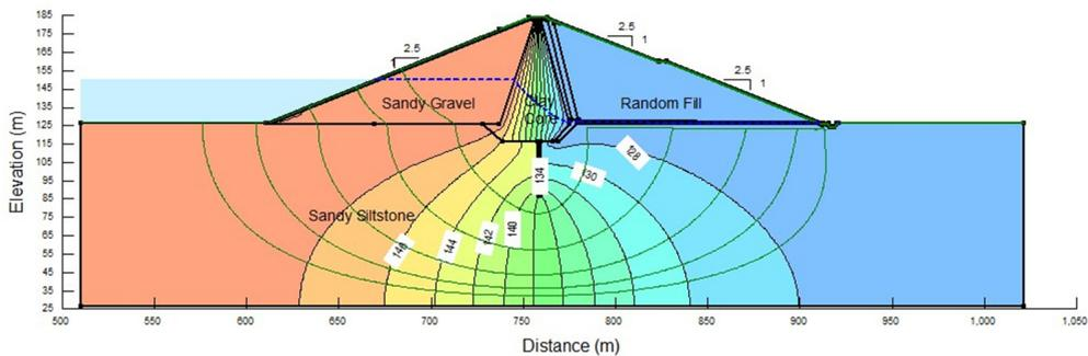
Fig. 4. Flow net of the selected section at normal reservoir level (150m).
