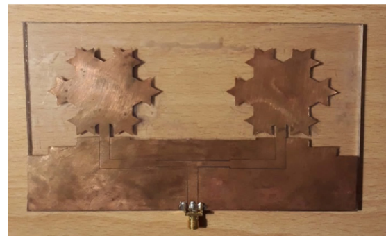
Fig. 11. The fabricated antenna array.
