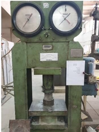
Fig. 3. Compressive strength measuring equipment.
