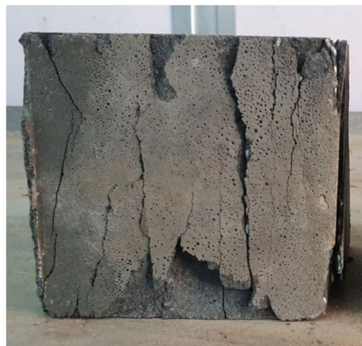
Fig. 7. Sample for tested for compressive strength after failure.
