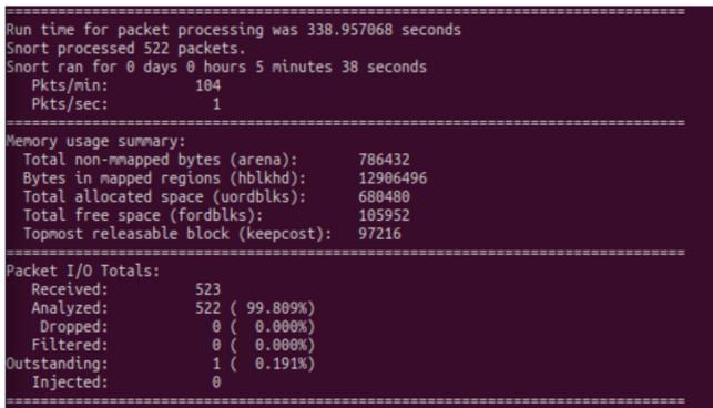
Fig. 4. Snort IDS platform analyzing packets.
