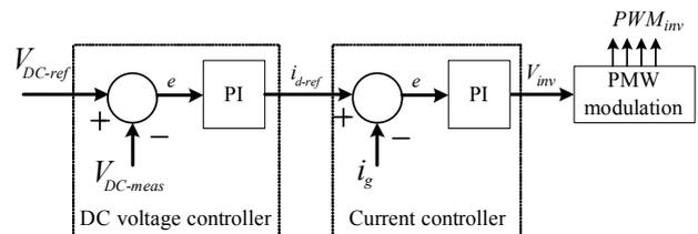
Fig. 4. Controllers for the hybrid grid-tie inverter.
