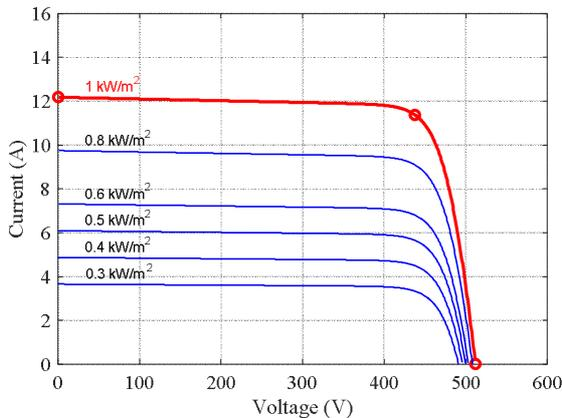
Fig. 2. Irradiance effect on the I-V curve.
