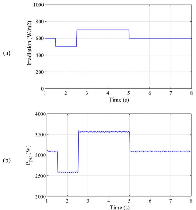
Fig. 9. Responses of the studied system with changing irradiance. (a) Irradiation, (b) active power of the solar PV system.
