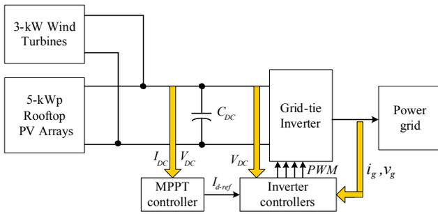
Fig. 1. Block diagram of the studied system.
