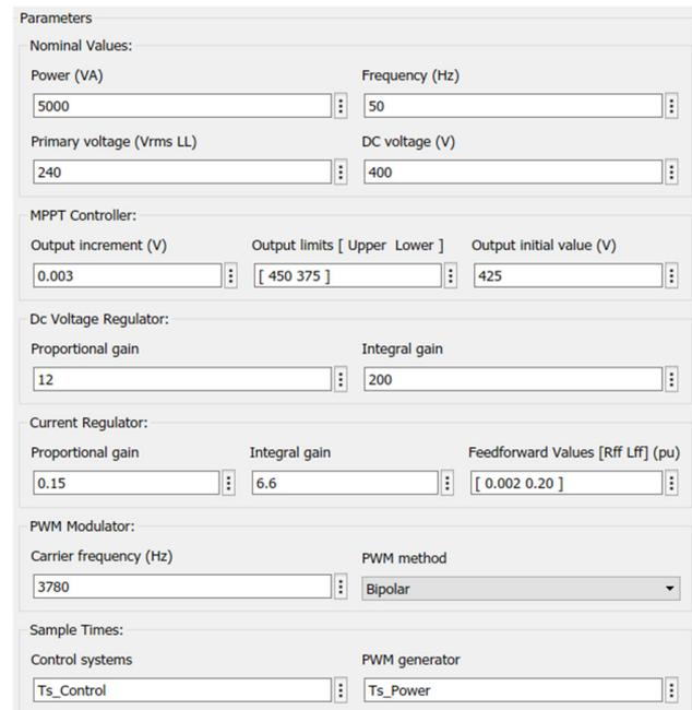
Fig. 8. Parameters of the inverter control block using the PI controller.
