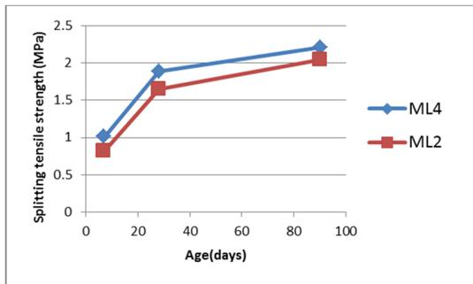
Fig. 5. Splitting tensile strength at 7, 28, and 90 days.
