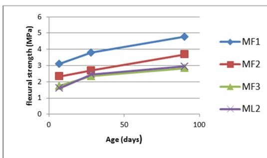
Fig. 6. Flexural strength at 7, 28, and 90 days.
