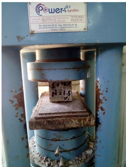
Fig. 2. Compressive strength test.
