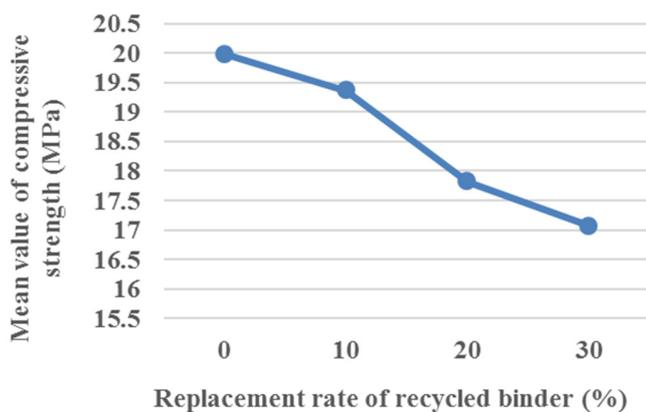
Fig. 3. Compressive strength of concrete at various replacement rates of recycled binder.
