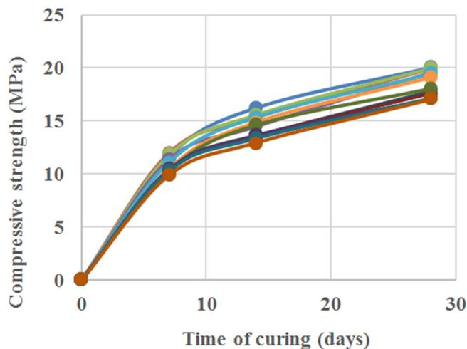
Fig. 4. The development of the compressive strength of concrete.
