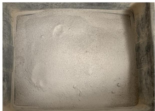
Fig. 1. Recycled fine-grained mixture obtained from crushed old concrete.
