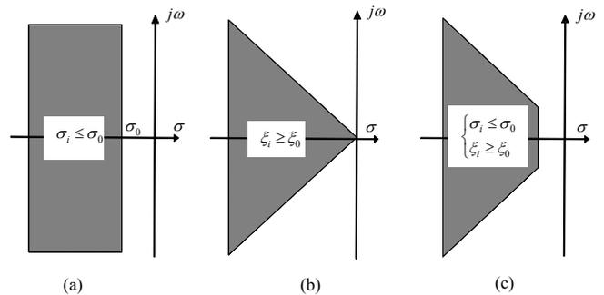
Fig. 2. Electromechanical modes location for different objective functions.
