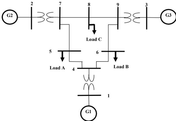
Fig. 4. Single line diagram of the WSCC system.
