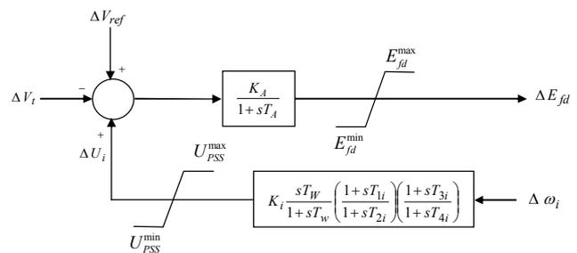
Fig. 1. IEEE type-ST1 excitation system with PSS.
