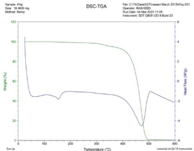
Fig. 4. FDSC and TGA analysis of sPP/S-4.
