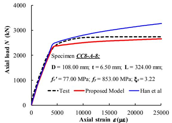
Fig. 7.  $N - \epsilon$  curves of CFST column with  $21.7 \leq D/t \leq 150$ .
