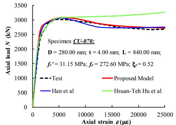
Fig. 6.  $N - \epsilon$  curves of CFST column for normal specimens.
