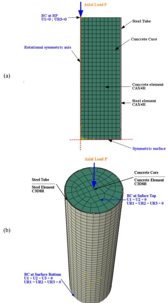
Fig. 3. Modeling of a CFST column. (a) Axisymmetric model, (b) full 3D model.
