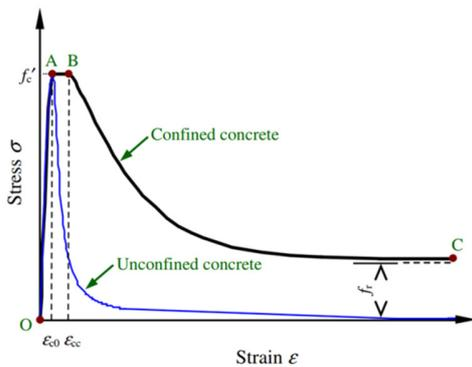
Fig. 2. The constitutive model of confined concrete.
