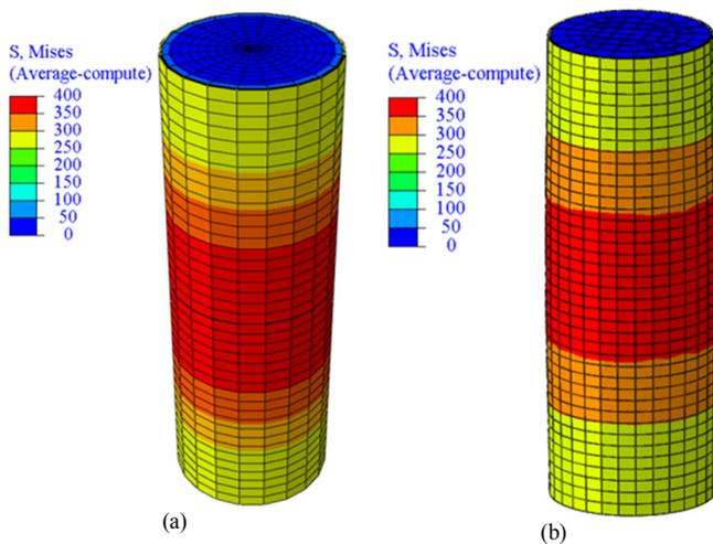
Fig. 4. Stress distribution of different models. (a) Axisymmetric model, (b) full 3D model.
