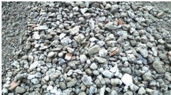
Fig. 2. Recycled coarse aggregates.
