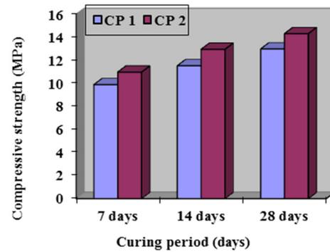
Fig. 5. Comparison of the strength of the two experimental recycled concrete mixes.
