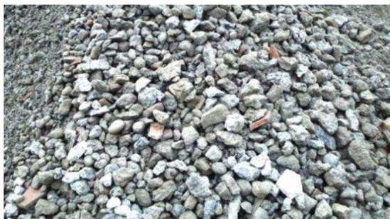
Fig. 2. Recycled coarse aggregates.
