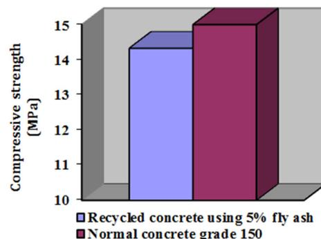
Fig. 6. Comparison of the strength of recycled concrete using fly ash with the conventional concrete.
