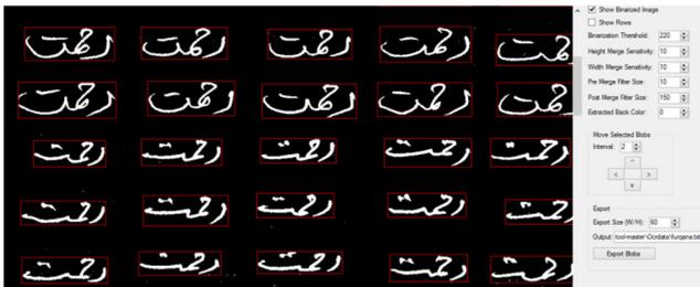
Fig. 2. OCR helper tool for cropping and binarization.
