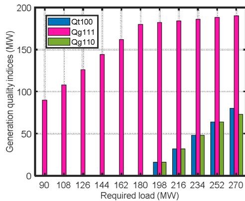
Fig. 4. Variation of generation capacity indices  $Q_{t100}$ ,  $Q_{g111}$ , and  $Q_{g110}$  with the variation of required load levels of the Wadi Aldawasir network.
