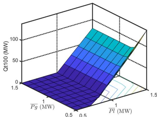
Fig. 5. 3-D graph of the variation of  $Q_{t100}$  with the required load levels and the available generation capacity levels of the Wadi Aldawasir network.
