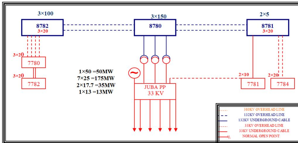
Fig. 3. Single-line diagram of the Wadi Aldawasir network.
