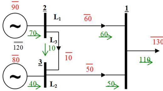
Fig. 2. The 3-bus sample power system.
