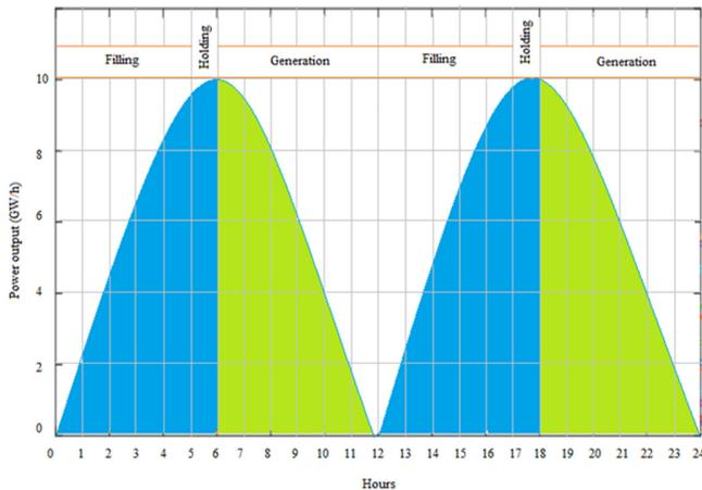
Fig. 1. A simple cycle of power generation.
