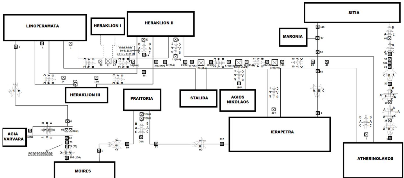
Fig. 2. Schematic of the Transmission System of Eastern Crete. Dotted lines depict underground cables. Legal numbering of towers is given within parentheses when different from the operational numbering. Larger squares denote double circuit towers that support three circuits. Linoperamata and Atherinolakos are step up substations. The line connecting Heraklion II to the Linoperamata-Ierapetra line is referred to as System-Heraklion II.
