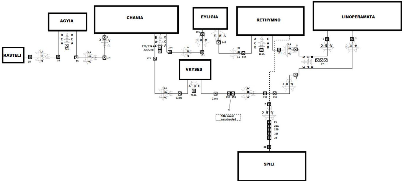
Fig. 1. Schematic of the Transmission System of Western Crete. Dotted lines depict underground cables. Chania and Linoperamata are step-up substations. The Linoperamata-Rethymno-Eyligia-Chania line is referred to as Linoperamata-Chania I and the Linoperamata-Vryses-Chania line as Linoperamata-Chania II.
