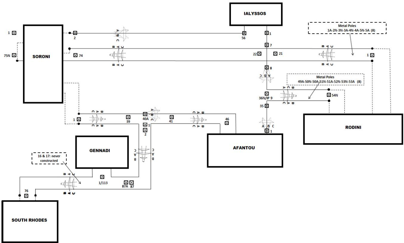
Fig. 3. Schematic of the Transmission System of Rhodes. Dotted lines depict underground cables. South Rodes and Soroni are step-up substations.
