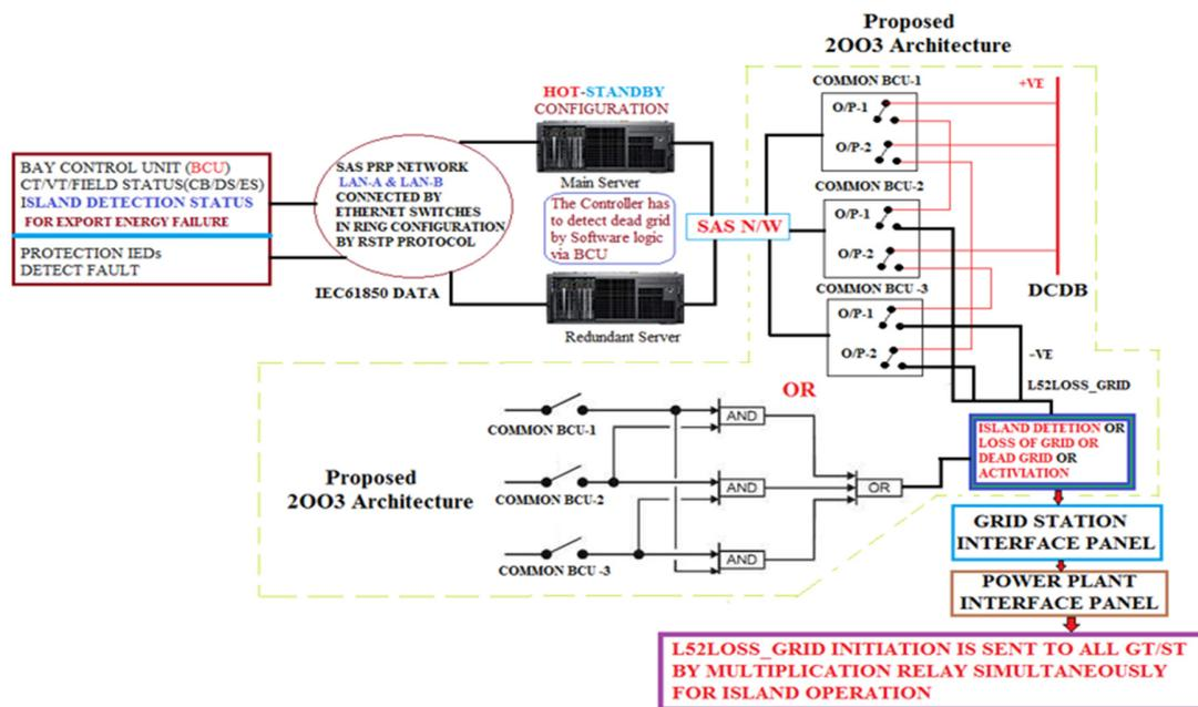
Fig. 2. The proposed 2oo3 communication architecture.
