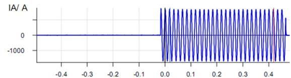
Fig. 11. P546 IED line current before and after fault.
