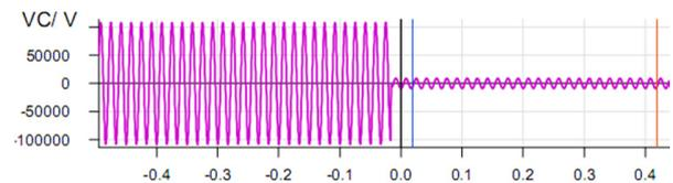
Fig. 10. P546 IED line voltage before and after fault.
