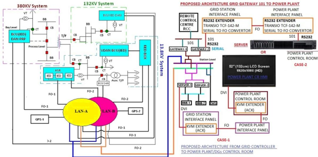
Fig. 4. SAS architecture with SLD using PRP, Non-PRP, and HSR for the proposed communication of the grid controller with the power plant.
