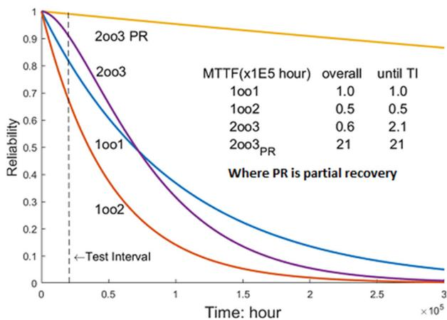
Fig. 3. Reliability functions for 1oo1, 1oo2, and 2oo3 without/with partial recovery (2oo3 and 2oo3-PR).
