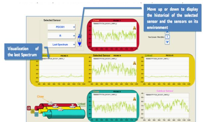
Fig. 6. Spectra acquired on the selected sensor.
