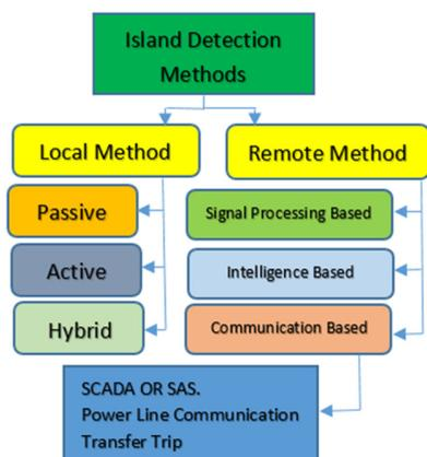
Fig. 1. Classification of island detection methods.
