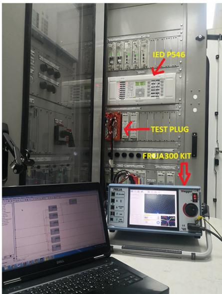
Fig. 8. Real-time experimental test bed for island fault simulation.
