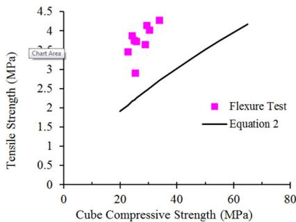
Fig. 8. Relationship between tensile and cube compressive strength.
