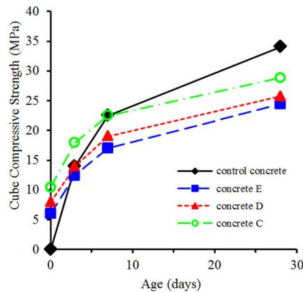
Fig. 6. Effect of maximum temperature holding time on concrete strength.
