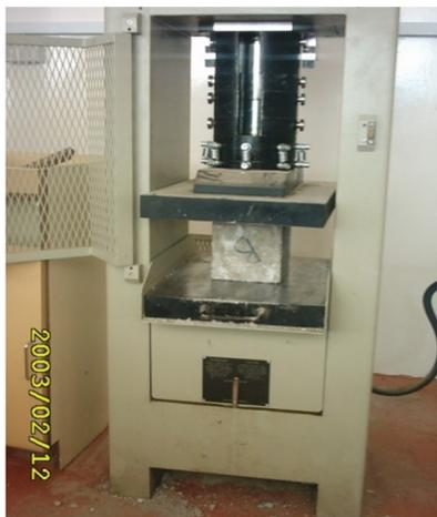
Fig. 2. The cube compressive strength test.
