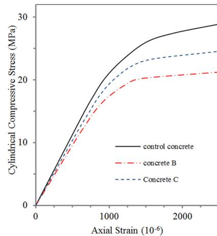
Fig. 9. Stress-strain curves for concretes in compression.
