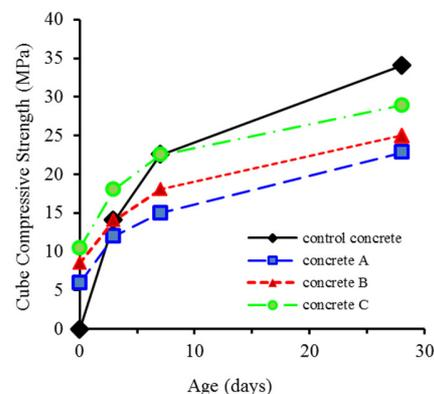
Fig. 3. The effect of the delay period on concrete strength.
