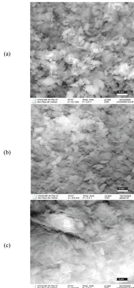
Fig. 9. SEM images of (a) gibbsite  $\text{Li}(\text{OH})_3$ , (b) intercalation of the lithium salt into gibbsite, and (c) precursor+stearic acid.
