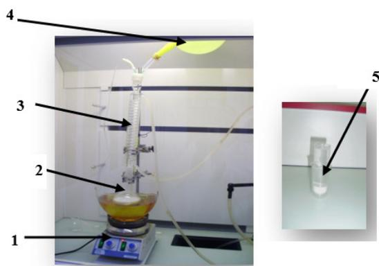
Fig. 1. Experimental setup of the gibbsite synthesis by lithium salt: 1: hotplate, 2: synthesis balloon, 3: refrigerant, 4: nitrogen gas balloon, 5: sample after filtration.
