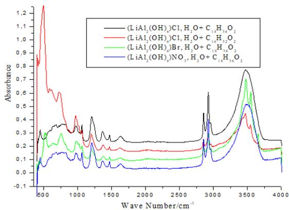
Fig. 8. IR spectra of gibbsite intercalated by Br,  $\text{NO}_3$  salts and exchanged by stearic and palmitic acid.
