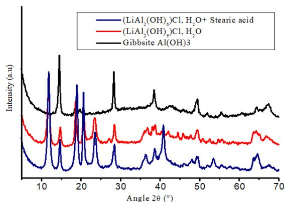
Fig. 3. X-ray diffraction (XRD) of crystalline gibbsite, gibbsite intercalated by LiCl, and anionic exchange precursor with fatty acids (stearic acid).
