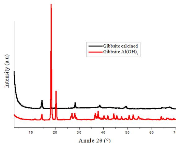
Fig. 2. X-ray diffraction (XRD) of crystalline gibbsite and gibbsite calcinated at  $300^\circ\text{C}$ .
