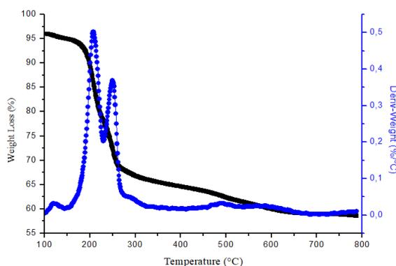
Fig. 5. TGA and DTG curves of  $[\text{LiAl}_2(\text{OH})_6]\text{Cl}\cdot\text{H}_2\text{O}$  precursor.
