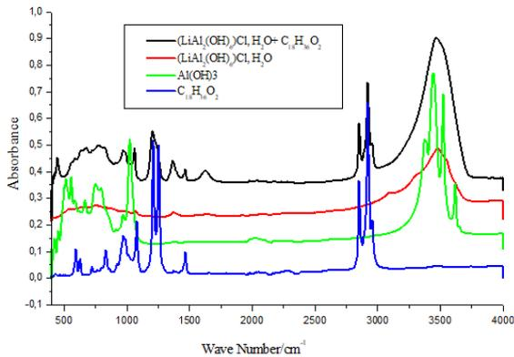
Fig. 7. IR spectra of gibbsite intercalated by salt and exchanged by stearic acid.
