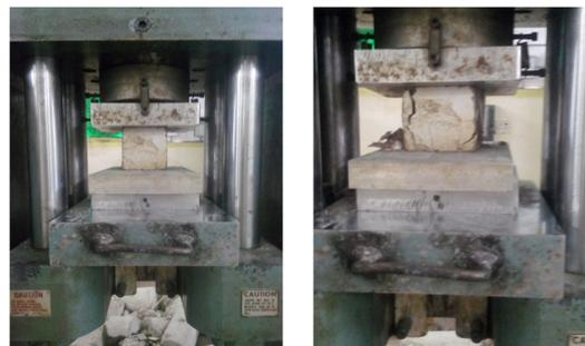
Fig. 2. A cubic specimen before and after compression testing.
