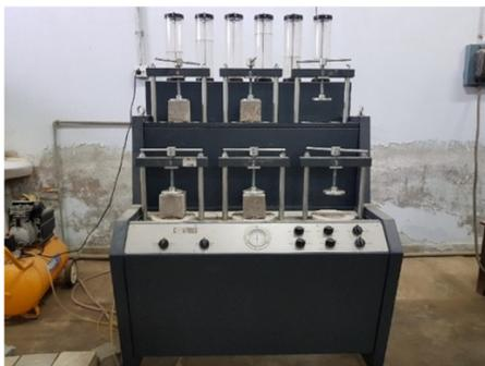
Fig. 4. Apparatus used for water penetration depth measurements.
