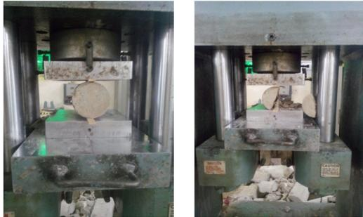
Fig. 3. A cylindrical specimen before and after tensile testing.
