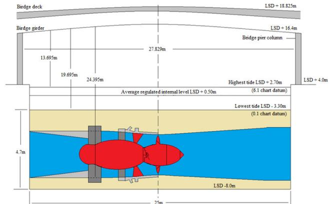
Fig. 4. Schematic diagram of one gate of bulb turbine for Kuching Barrage.
