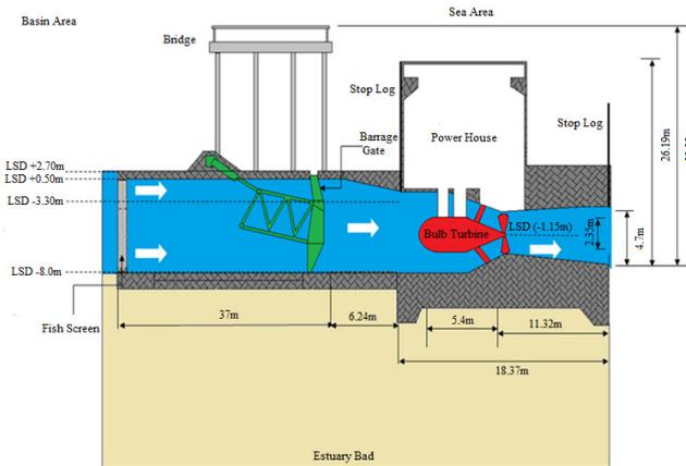
Fig. 2. Powerhouse layout of Kuching Barrage tidal energy plant.
