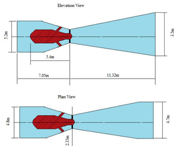
Fig. 1. Kuching Barrage tidal energy plant powerhouse dimensions.
