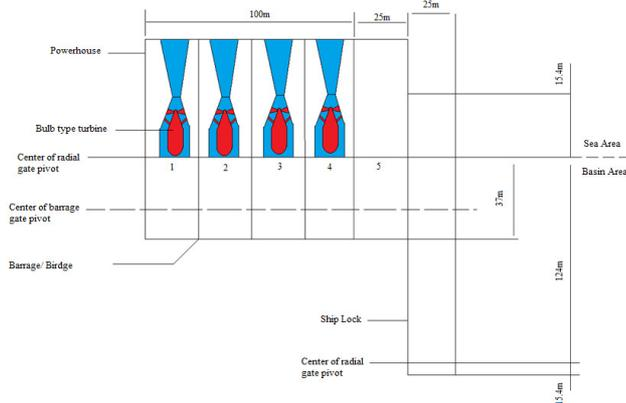
Fig. 3. Plan view of Kuching Barrage tidal range energy plant scheme at four gates.
