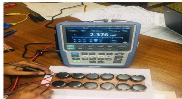
Fig. 7. Super capacitor bank.
