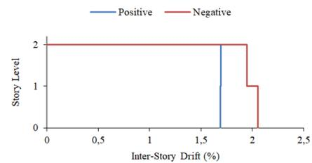
Fig. 15. 80% excitation of the 1994 Northridge earthquake.
