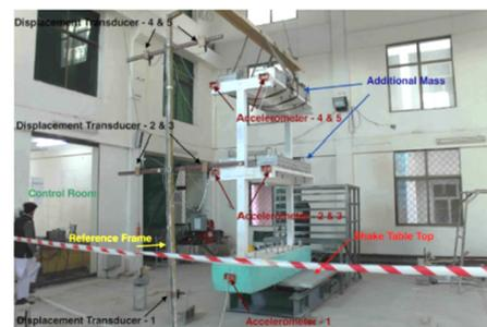
Fig. 5. Instrumentation plan of the test specimen.
