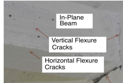
Fig. 23. Distribution of cracks beam (in-plane).
