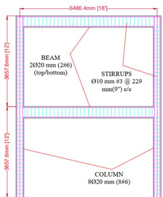
Fig. 2. Prototype elevation and structural detailing.
