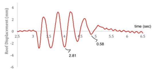
Fig. 8. Free vibration test for calculation of damping.
