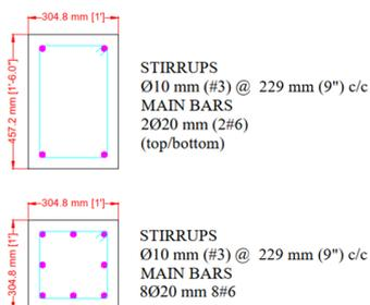
Fig. 3. Beam and column section detailing (prototype).
