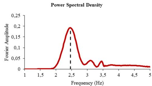
Fig. 7. Fundamental frequency of the test specimen.
