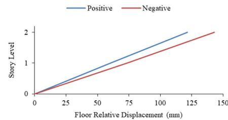
Fig. 19. 80% excitation of the 1994 Northridge Earthquake.
