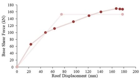
Fig. 21. Capacity curve of the tested specimen under shake table testing.
