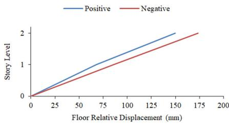
Fig. 20. 100% excitation of the 1994 Northridge earthquake.
