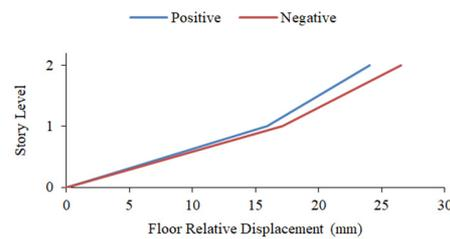
Fig. 17. 20% excitation of the 1994 Northridge earthquake.
